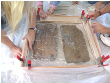
REMOVING MOLD BOX
