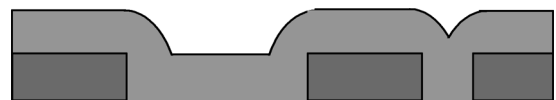
Figure 1. A large gap between two features on the lower layer (dark gray) results in topography in the upper layer (light gray) equal to the thickness of the lower layer, whereas a small gap results in much smaller topography.
