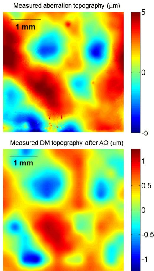
**Fig. 10.** Comparison of the wavefront shapes roughly at the same location of (top) the phase screen and (bottom) the DM after conjugate AO with full-image contrast correction [i.e., same as in Fig. 8(b)]. In both cases, the wavefront shapes were measured with a Zygo white-light interferometer.
