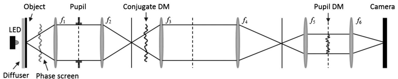
**Fig. 6.** Experimental setup. Lens focal lengths are  $f_1 = 100$  mm,  $f_2 = 100$  mm,  $f_3 = 100$  mm,  $f_4 = 200$  mm,  $f_5 = 75$  mm, and  $f_6 = 50$  mm. Solid vertical lines correspond to object planes; dashed vertical line correspond to pupil planes. Note that in reality the DMs are reflective and the layout was doubly folded.
