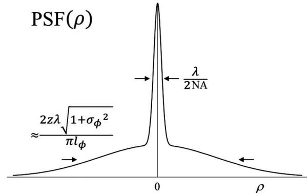
Fig. 3. Example of an effective PSF ( $\rho$ ) after degradation by a phase screen. The initial diffraction-limited PSF ( $\text{PSF}_0$ ) is reduced by a factor  $e^{-\sigma_{\phi}^2}$  and rides on a broader blurred background of power  $1 - e^{-\sigma_{\phi}^2}$ .
