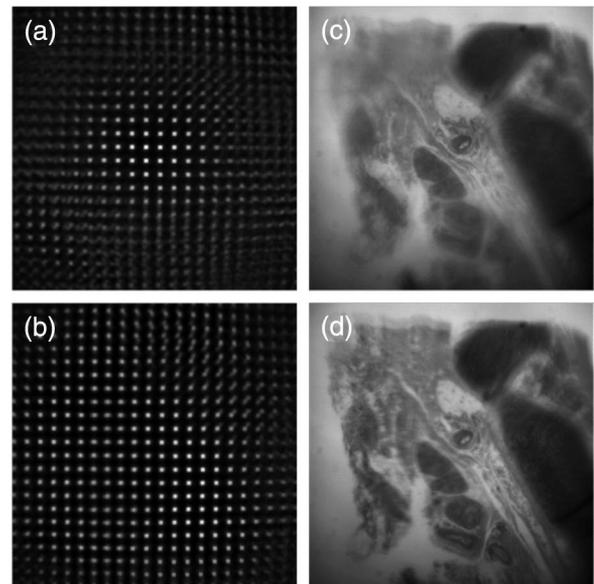
**Fig. 8.** Experimental results for conjugate AO. Images of aperture array after AO correction that optimized contrast in a zone about the origin of size (a)  $250\ \mu\text{m} \times 250\ \mu\text{m}$  (single guide star), and (b)  $4\ \text{mm} \times 4\ \text{mm}$  (entire image). (c) and (d) are corresponding images of tissue section.
