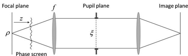
Fig. 1. Basic microscope layout.
