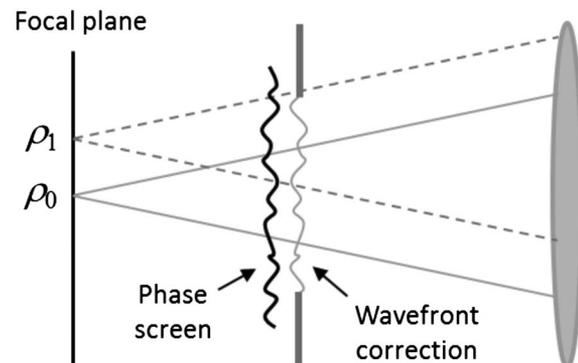
**Fig. 5.** Interpretation of what defines FOV for conjugate AO. The fixed wavefront correction cancels the aberrations caused by the fixed phase screen. The FOV is then limited by size of the projected DM itself, albeit with blurred edges dependent on distance  $z$  of the phase screen and the microscope NA.
