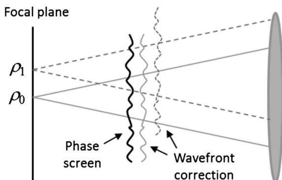
**Fig. 4.** Interpretation of what defines FOV for pupil AO. As an object point  $\rho_1$  becomes displaced from the guide-star point  $\rho_0$ , its wavefront correction becomes uncorrelated with the fixed phase-screen aberrations, and AO fails.
