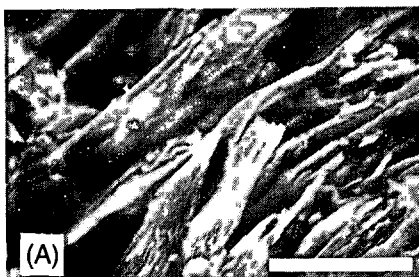
Fig. 9. Chips of (A) germanium machined at 1.5\text{-}\mu\text{m} feed, 0.5\text{-}\mu\text{m} depth of cut, and 0.025\text{-}\mu\text{m} t_m and (B) copper machined at 6.3\text{-}\mu\text{m} feed, 2.3\text{-}\mu\text{m} depth of cut, and 0.5\text{-}\mu\text{m} t_m . (bars = 5 \mu\text{m} )
