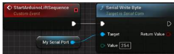
Figure 33: Simple call mechanism to trigger lift action
