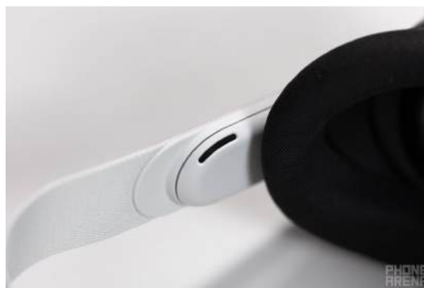
Figure 27: Speaker placement on the Meta Quest 3
