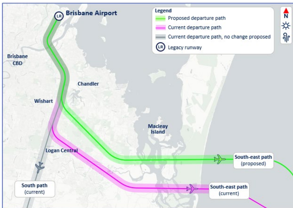
Figure 2: Current (pink) south and south-east departure paths and proposed (green) south-east departure path, with 1km buffers either side. No change proposed for grey section of south path.
