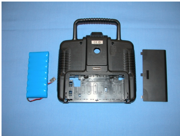
Photo 5 Cover and battery removed
