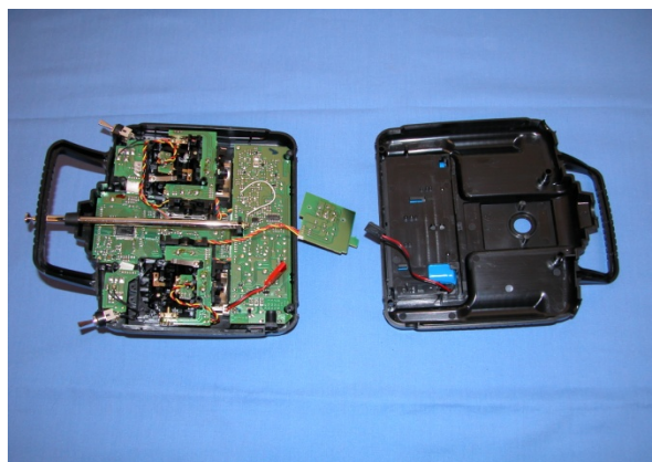
Photo 4 Trainer PCB & battery lead removed
