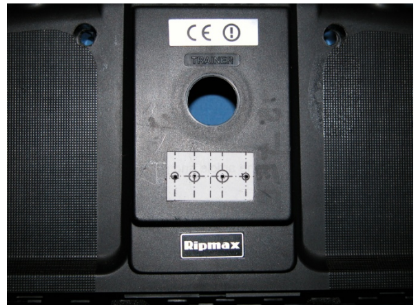
Photo 6 Drilling template fixed into position
