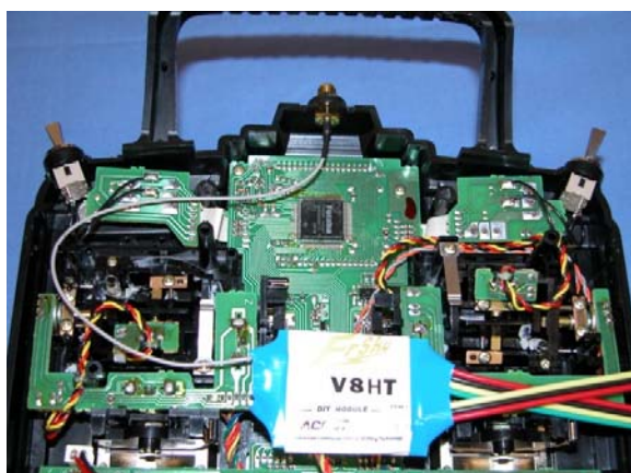
Photo 10 Aerial connector in position
