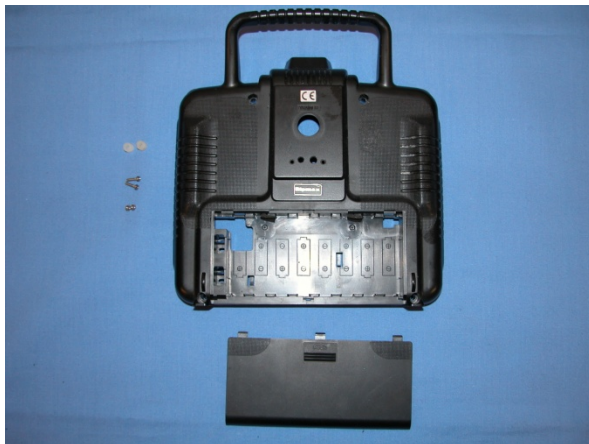
Photo 7 Holes drilled in back of case
