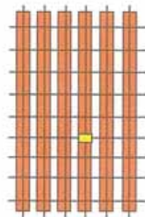
Fig 4 Strip Board - track cutting
