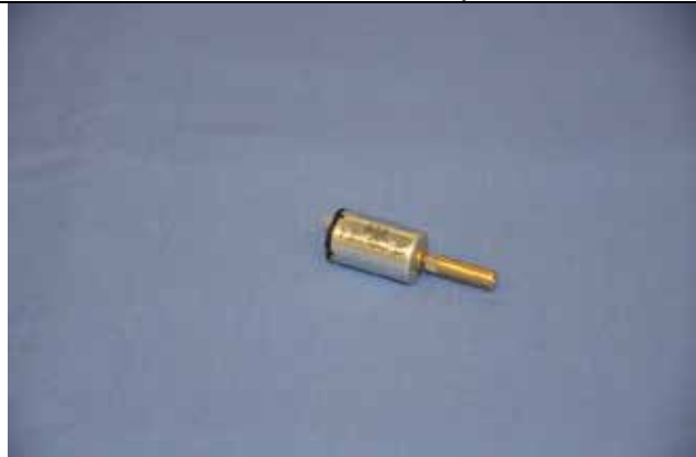
Photo 13 Motor and Coupling Bonded
