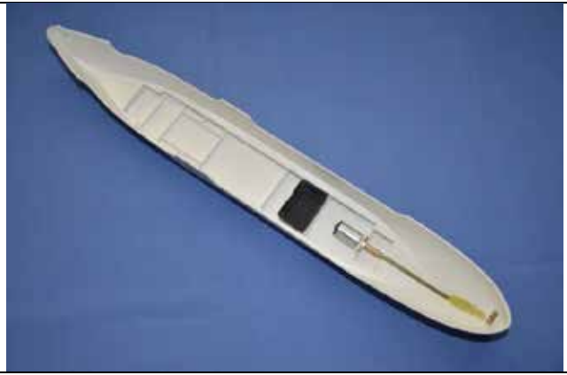
Photo 17 ESC housing, Receiver Compartment, Switch & Servo Bracket
