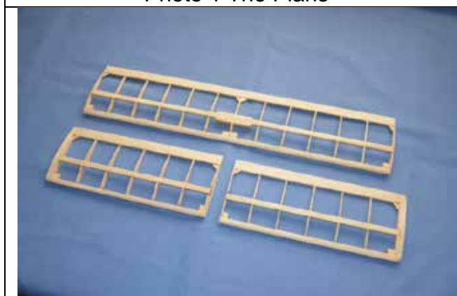
Photo 3 Main Wing Assemblies
