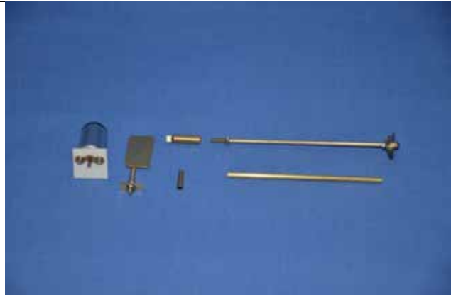
Photo 11 Rudder and Propeller Shaft
