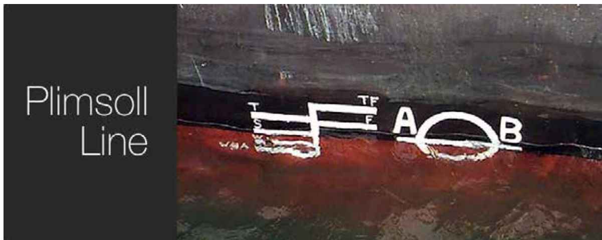
Plimsoll mark on a floating ship
