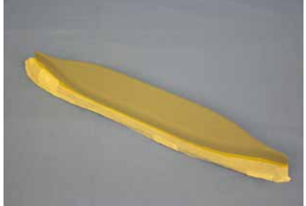
Photo 20 Hull Masked and Primed
