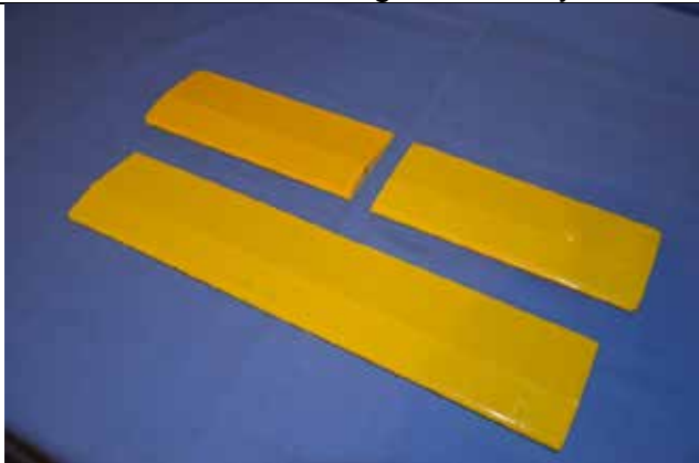
Photo 7 Main Wing Assemblies Covered
