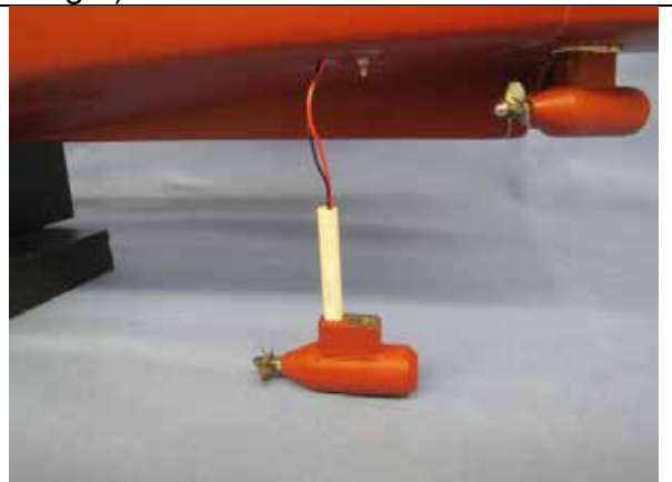
2 POD lowered from the Hull
