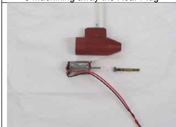
5 Motor & Loose Shaft Extracted
