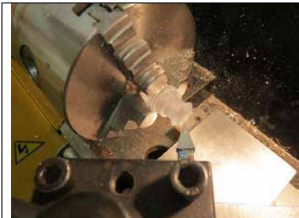
9 Machining the new End Cap
