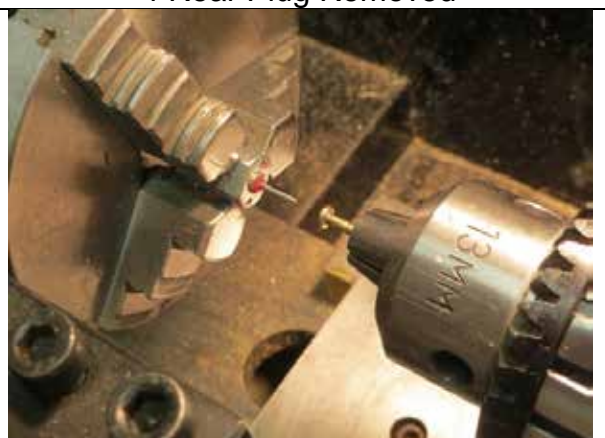
6 Shaft Aligned ready for Bonding
