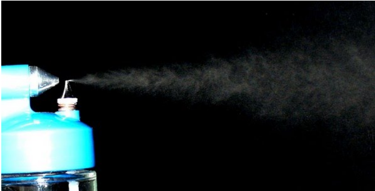
Badger 250 airbrush in use (using water) to show the spread of spray.
