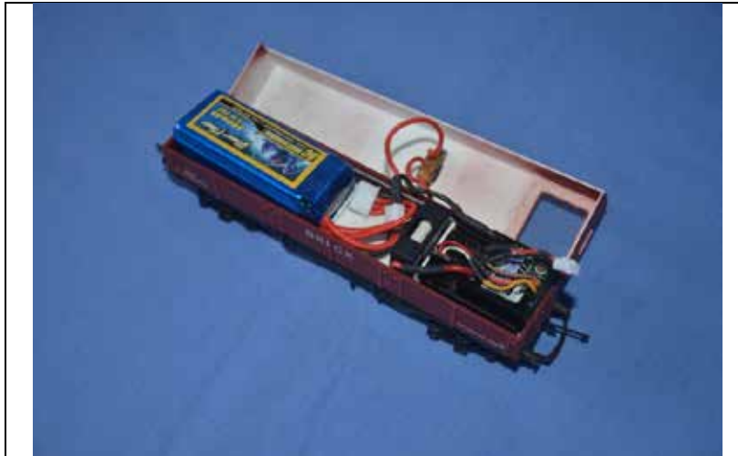
Photo 10. Wagon with Battery, Radio Receiver & ESC
