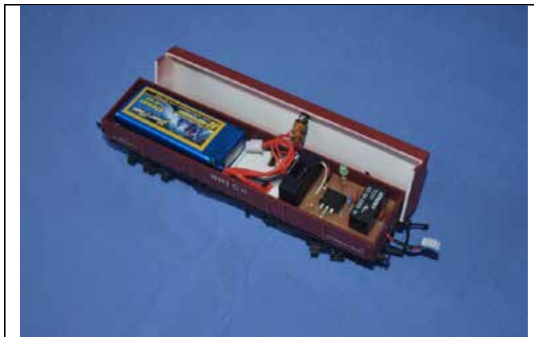
Photo 6 Wagon with Battery & Hall Switch Fitted
