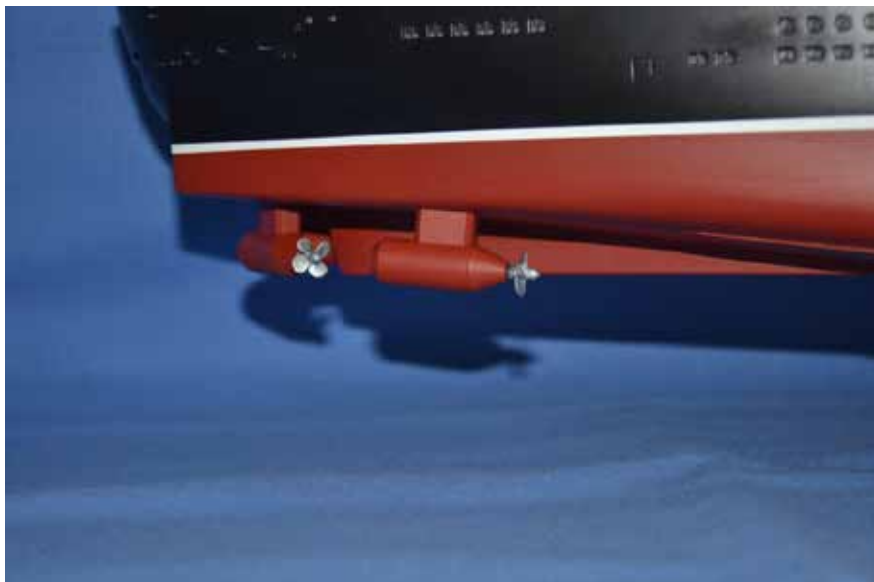
Photo 04: The POD installed
