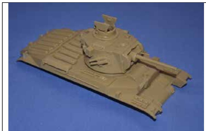
Photo 15 Upper Hull Assembly Complete
