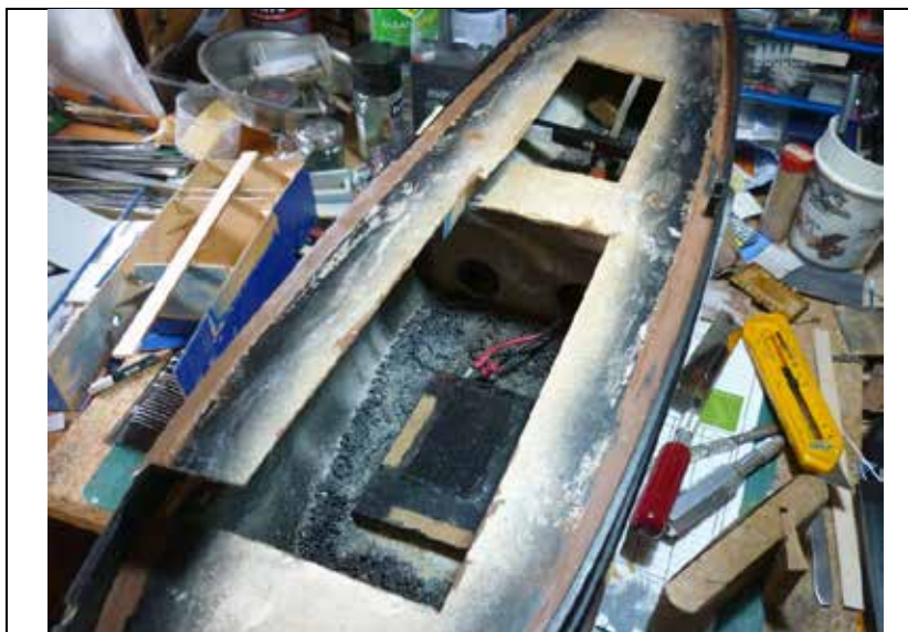
Photo 04 Deck Being Removed
