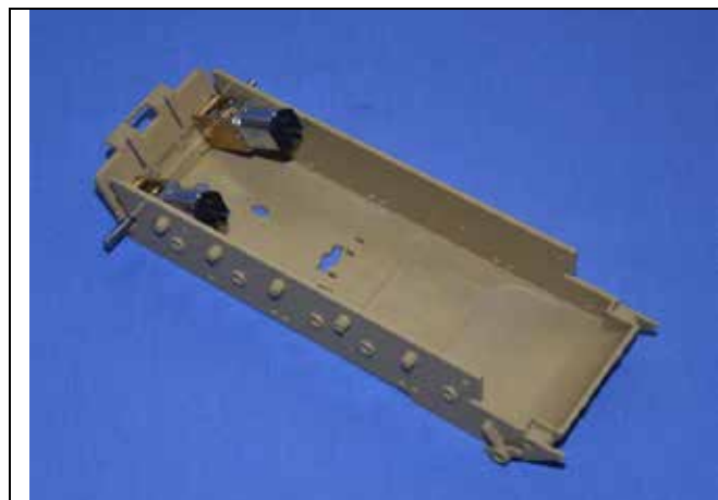
Photo 12 Motor Gear box's Fitted
