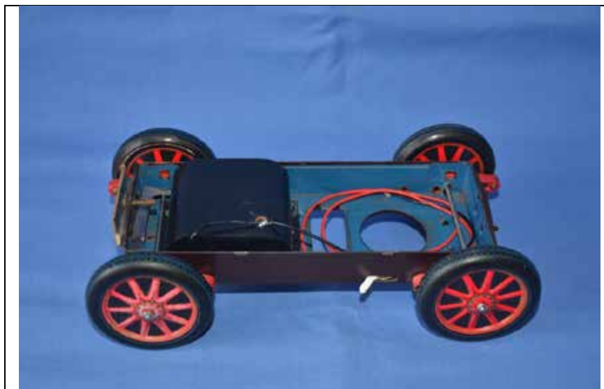
Photo 06 Battery Box and Power Switch Fitted
