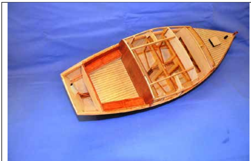
Photo 17. Seating Cut to Size and Bonded into Position
