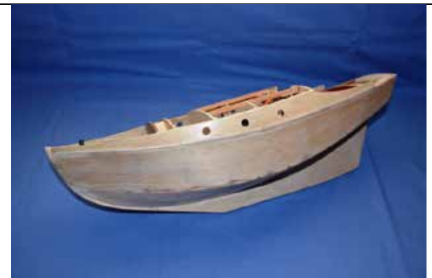
Photo 22. Cabin Sides Fitted
