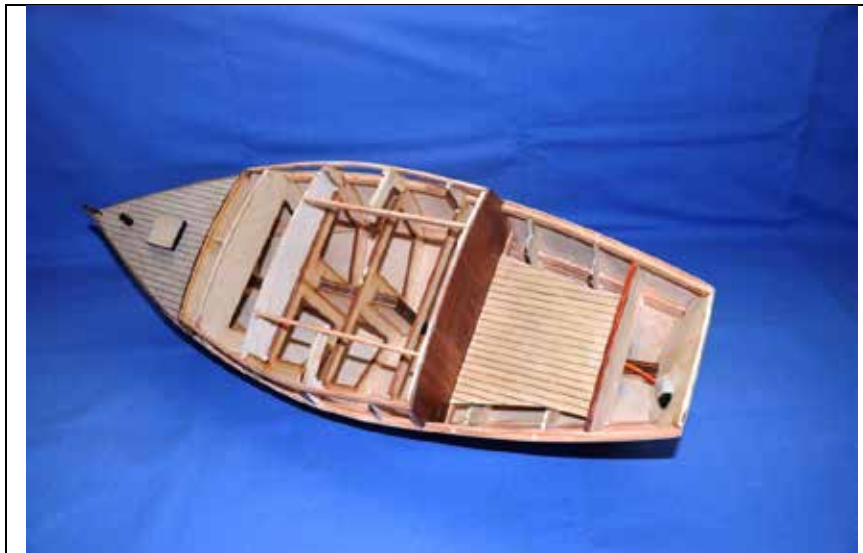
Photo 16 Well Deck Fitted in Position
