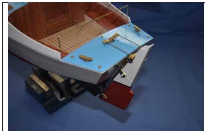
Photo 34 Main Sail Horse and Rudder Fitted
