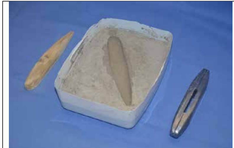
Photo 29 Male Plug, Female Mould and Cast Ballast Weights
