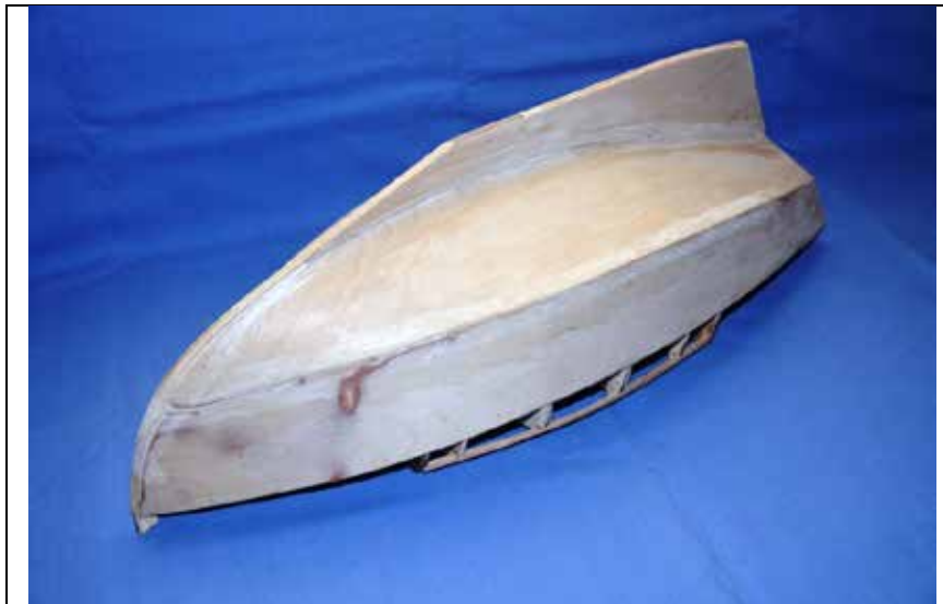
Photo 20. Hull Final Covering & Sanded
