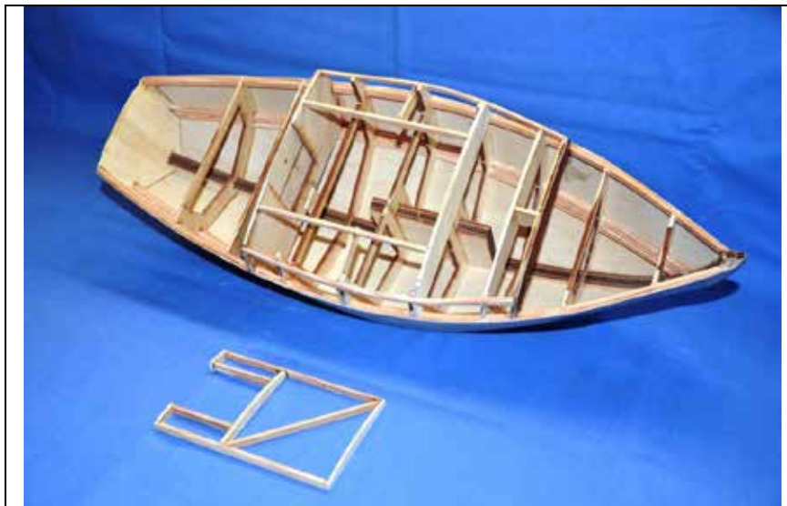
Photo 12 Cabin Roof Hatch Construction
