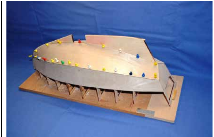
Photo 09. Hull Bottom Pinned and Glued into position
