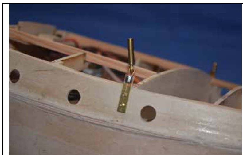
Photo 28. Turnbuckles Mounted to Cabin Sides
