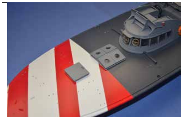
Photo 23 Foredeck Hatches Fitted
