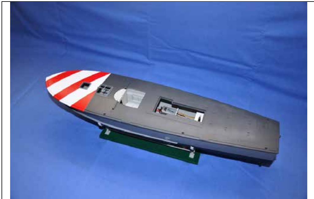
Photo 15 Deck Painted and Fitted to the Hull
