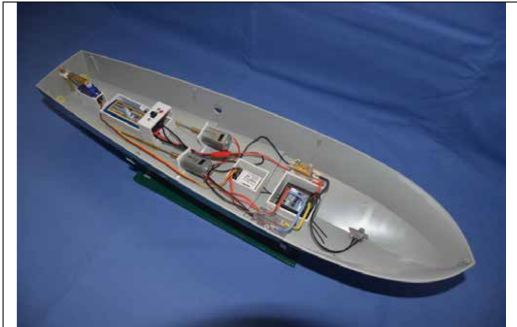
Photo 12 RC System Installed and Wired
