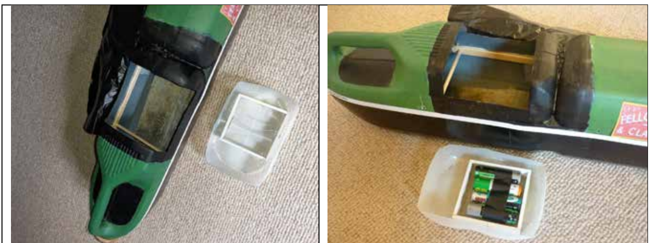
Cargo hold with bracing, lead ballast and removable cargo hold
