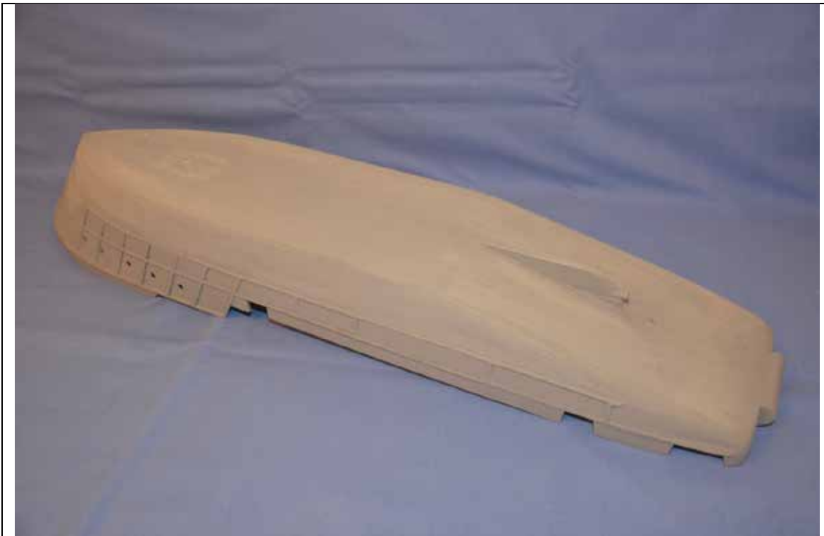
Photo 09: Hull stripped and primed
