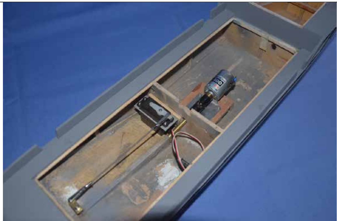
Photo 8: Motor and Rudder Servo installed
