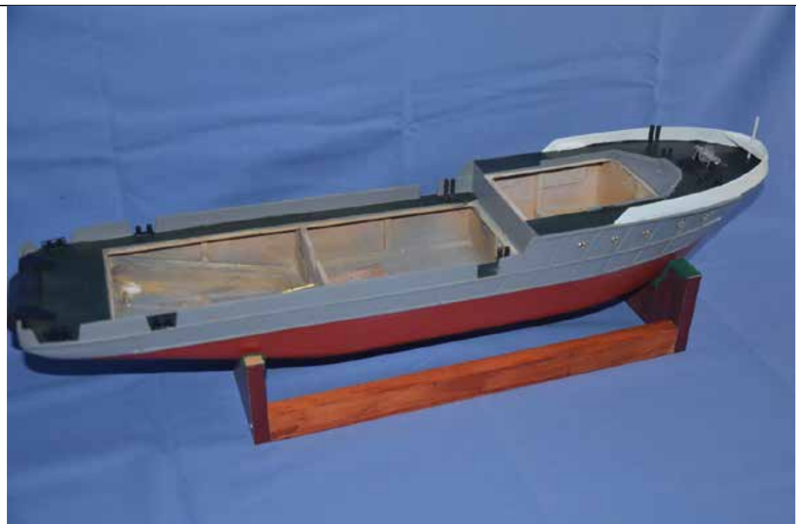
Photo 11: Decks & Bulwarks painted with the fittings added
