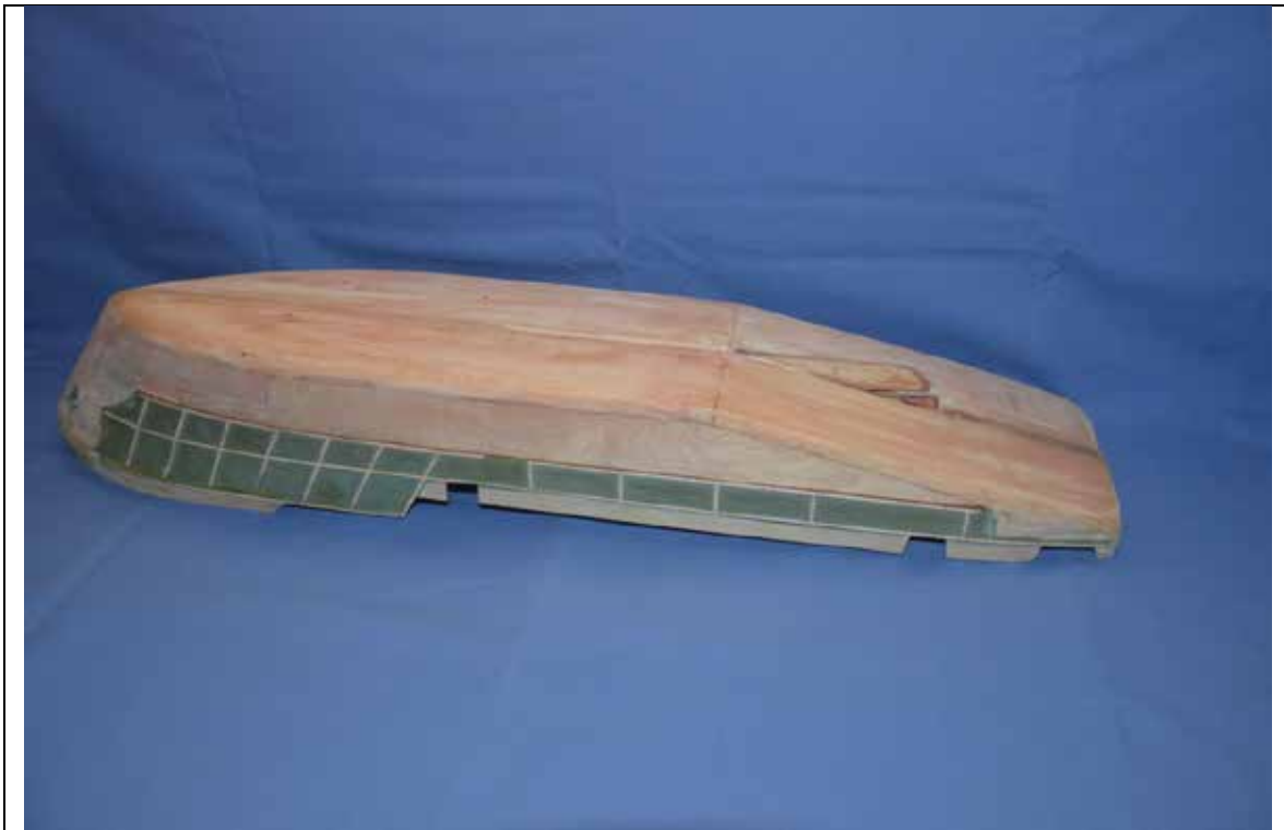
Photo 05: Hull stripped ready for painting
