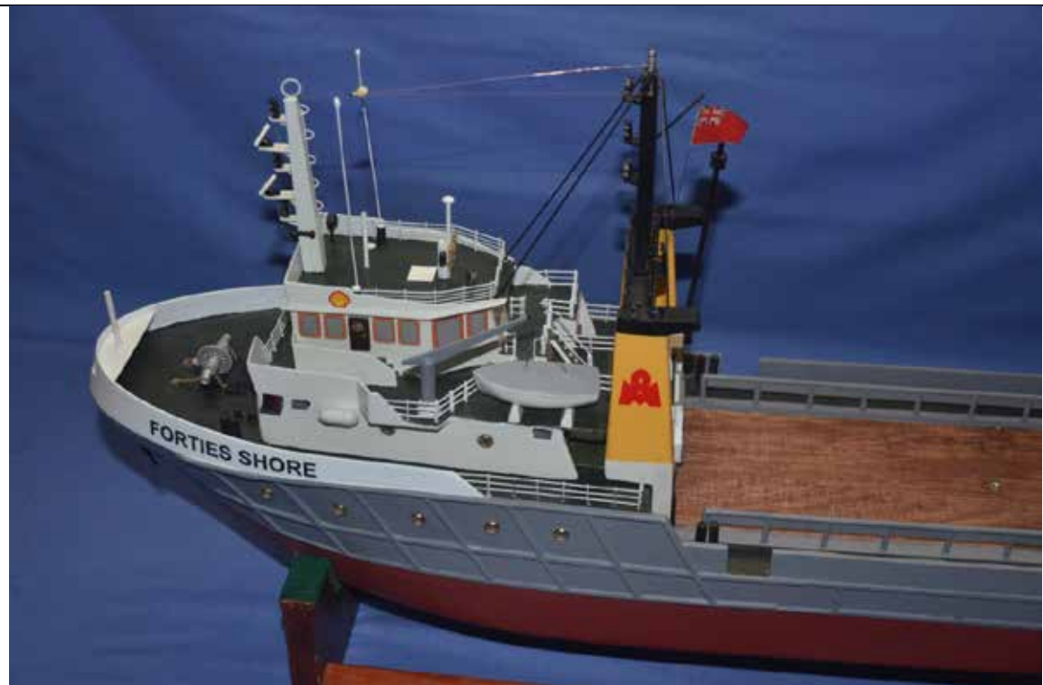
Photo 22 Masts and Life Boat Fitted
