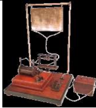
Fig 11 Early Marconi Experimental Transmitter
