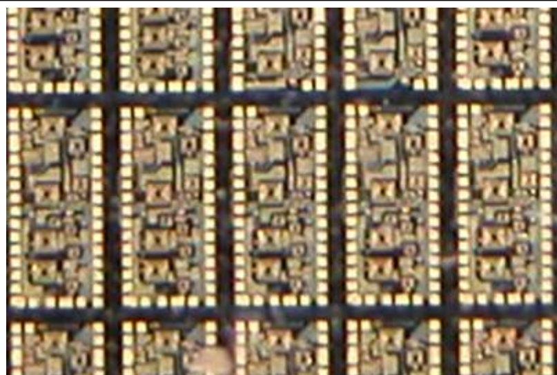
Fig 61 The Wafer magnified to show the individual IC's (actual size about 1x2.5mm)
