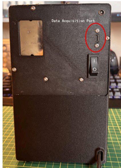
Figure 11. Data Acquisition / Device Reprogramming Port
