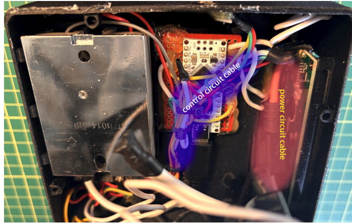
Figure 9. Separate wiring for dual power system
