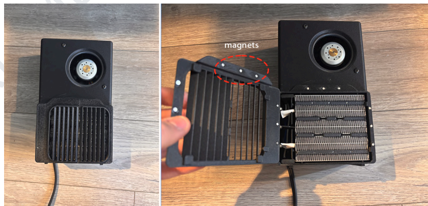
Figure 15. Deflector Installation Mechanism
