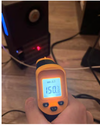
Figure E1. PTC Heater Surface Temperature
