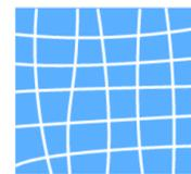
A traditional filter mesh may deform under high pressure and temperature, thus affecting the removal ratings.
