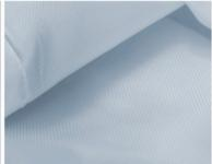
The structured set-up of the polyamide filter medium with modern Composite-Layer technology guarantees precise separation rates of 0.4 – 50 µm with a restraining efficiency of 99.9% (Beta 1000).
