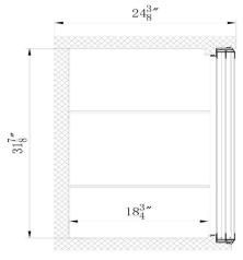
Rated Voltage 220 V Rated Frequency 50 Hz **Total Input Power** 284W 2.66A **Total Current Total Capacity** 11.23 cu ft 4-5 **Climatic Category Protection Type** Design Pressure High Side **385 PSIG 150 PSIG Design Pressure Low Side Insulation Blowing Gas C-Pentane** R290/3.17 oz Refrigerant
