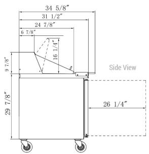
**Cutting Board Size** 29 x 9 Rated Voltage 220 V Rated Frequency 50 Hz **Total Input Power** 225W **Total Current** 2.0A **Total Capacity** 6.56 cu ft **Climatic Category** 4-5 **Protection Type** Design Pressure High Side 300 PSIG **150 PSIG Design Pressure Low Side** C-Pentane **Insulation Blowing Gas** R290/2.82 oz Refrigerant
