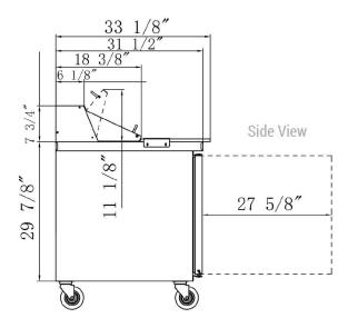
**Cutting Board Size** 60 x 14.5 Rated Voltage 220V Rated Frequency 50Hz **Total Input Power** 280W 2.4A **Total Current Total Capacity** 14.33 cu ft **Climatic Category** 4-5 **Protection Type 300 PSIG** Design Pressure High Side **Design Pressure Low Side 150 PSIG**
