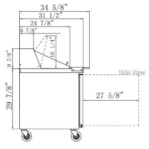
**Cutting Board Size** 60 x 9 Rated Voltage 220 V Rated Frequency 50 Hz **Total Input Power** 280W 2.4A **Total Current** 14.33 cu ft **Total Capacity Climatic Category** 4-5 **Protection Type** Design Pressure High Side **300 PSIG** Design Pressure Low Side **150 PSIG Insulation Blowing Gas C-Pentane** Refrigerant R290/3.88 oz 1/6 PAN COUNT: 24
