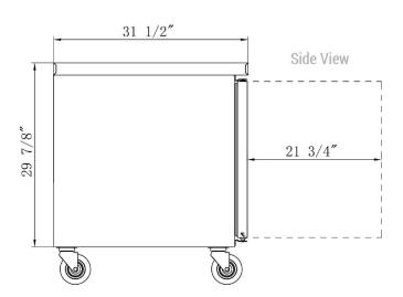
Rated Voltage 220 V Rated Frequency 50 Hz 660W **Total Input Power Total Current** 8.0A **Total Capacity** 12.21 cu ft **Climatic Category** 4-5 **Protection Type Design Pressure High Side 300 PSIG Design Pressure Low Side 150 PSIG** C-Pentane **Insulation Blowing Gas** Refrigerant R290/3.70oz
