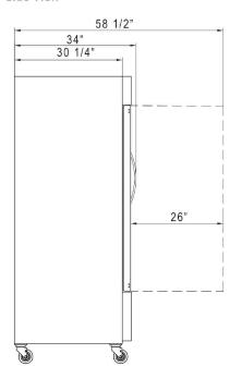
Rated Voltage 220V Rated Frequency 50Hz **Total Input Power** 550W **Total Current** 5.3A 8.1kW.h/24h **Energy Consumption Total Capacity** 17.79 cu ft **Climatic Category Protection Type** Design Pressure High Side **300 PSIG** Design Pressure Low Side **150 PSIG Insulation Blowing Gas** C-Pentane Refrigerant R290/4.41oz
