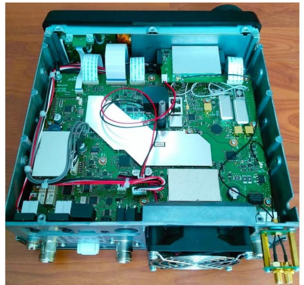
Pan Adapter kit installed in an ICOM 9700 transceiver for additional operational features.
