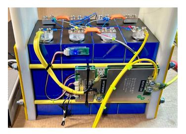
The battery pictured above was built by the Vilas County Amateur Radio Club at the meeting on Jan. 8th, 2025. It consists of 4 Lithium Iron Phosphate Prismatic cells "LiFePo4" (3.2 vdc each) connected in series to produce a 12-volt battery.
