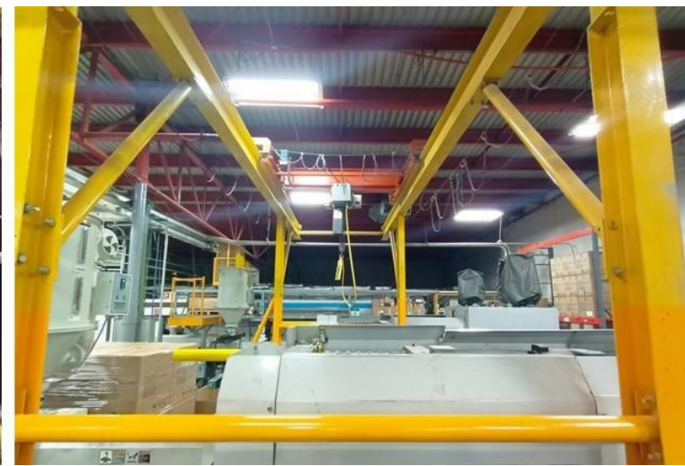
Electric Traveling crane, 3-ton capacity, 1 section of 20 ft.
