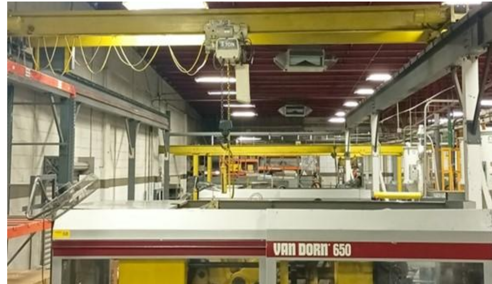
Electric Traveling Crane, 3-ton capacity, 3 sections of 20 ft each
