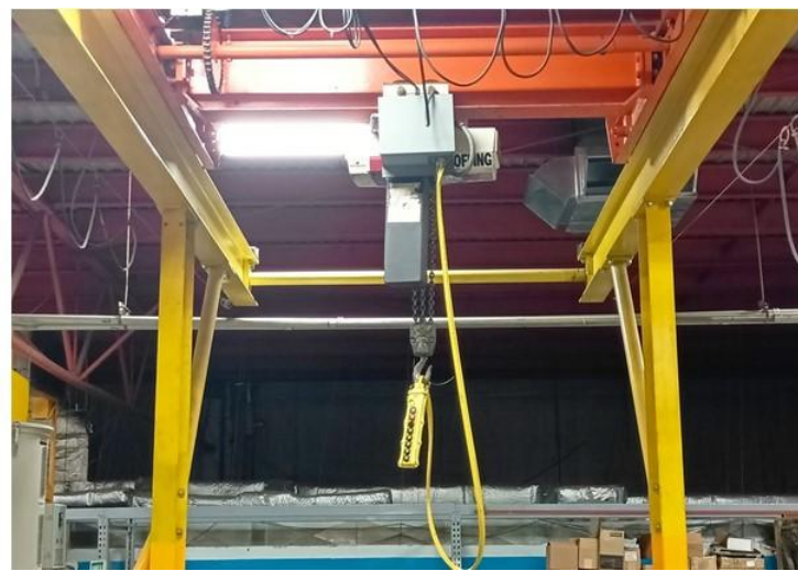
Electric Traveling crane, 3-ton capacity, 1 section of 20 ft.
