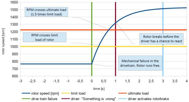
Rotor speed after a drivetrain failure, see attached spreadsheet for the calculations. Full page view at the end.
