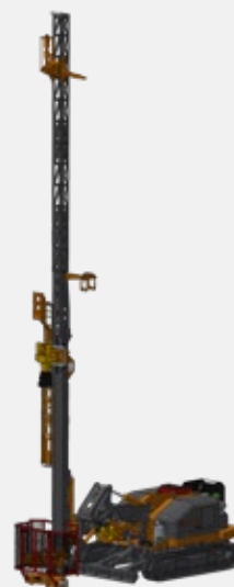
CONFIGURAZIONE JET GROUTING JET GROUTING CONFIGURATION
