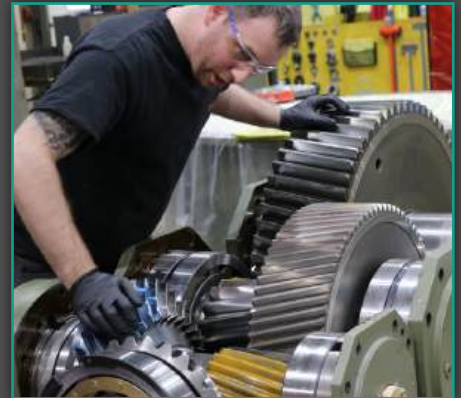
INDUSTRIAL GEARBOX MAINTENANCE
